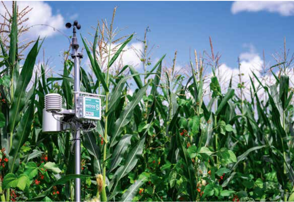
METOS 5: Smart IoT station integrating weather, soil, and crop sensors to deliver precise real-time insights
