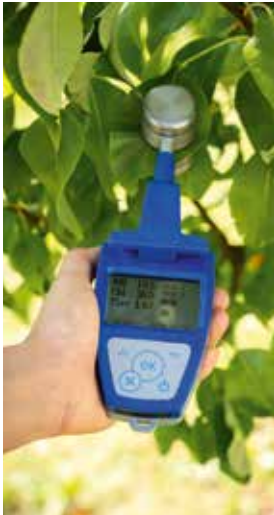
DUALEX: Leaf-clip sensor for instant, non-destructive measurement of chlorophyll and nitrogen status
