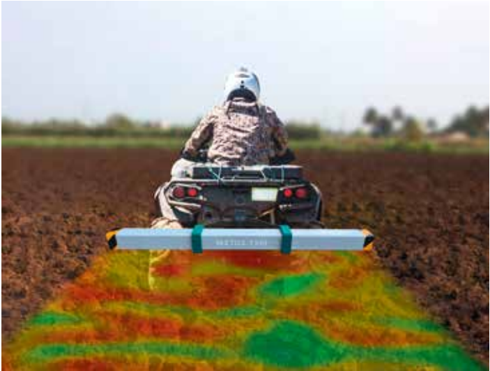
METOS TSM: Soil moisture monitoring wand mapping for precise irrigation and crop management
